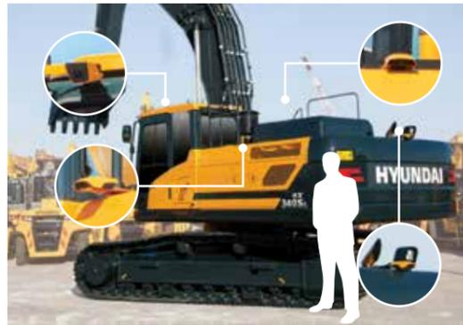
\*AVM (Around View Monitoring): Secure field of vision in all directions by nine views including 3D bird's eye view and 2D/4CH view.
